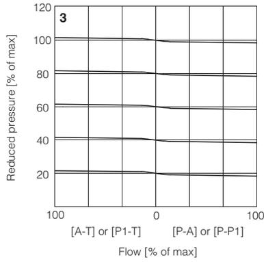
**11.3 Pressure drop/flow diagram**
