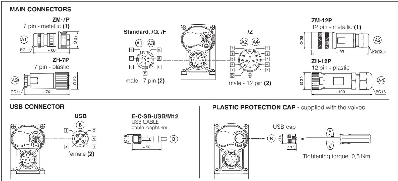
(1) Use of metallic connectors is strongly recommended in order to fulfill EMC requirements (2) Pin layout always referred to driver's view
