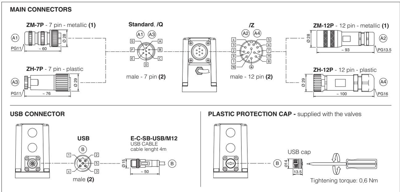
(1) Use of metallic connectors is strongly recommended in order to fulfill EMC requirements (2) Pin layout always referred to driver's view
