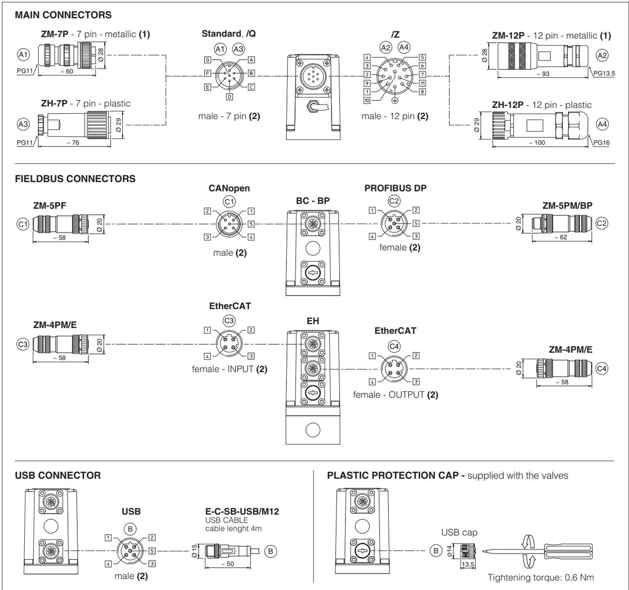
(1) Use of metallic connectors is strongly recommended in order to fulfill EMC requirements (2) Pin layout always referred to driver's view
