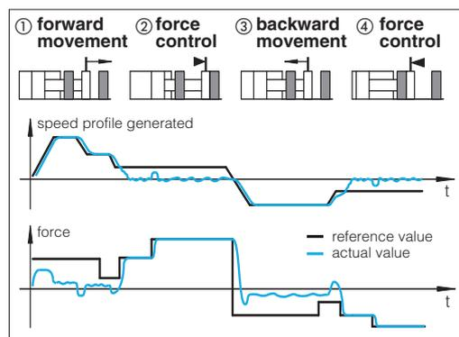
Alternated control configurations - software selectable
