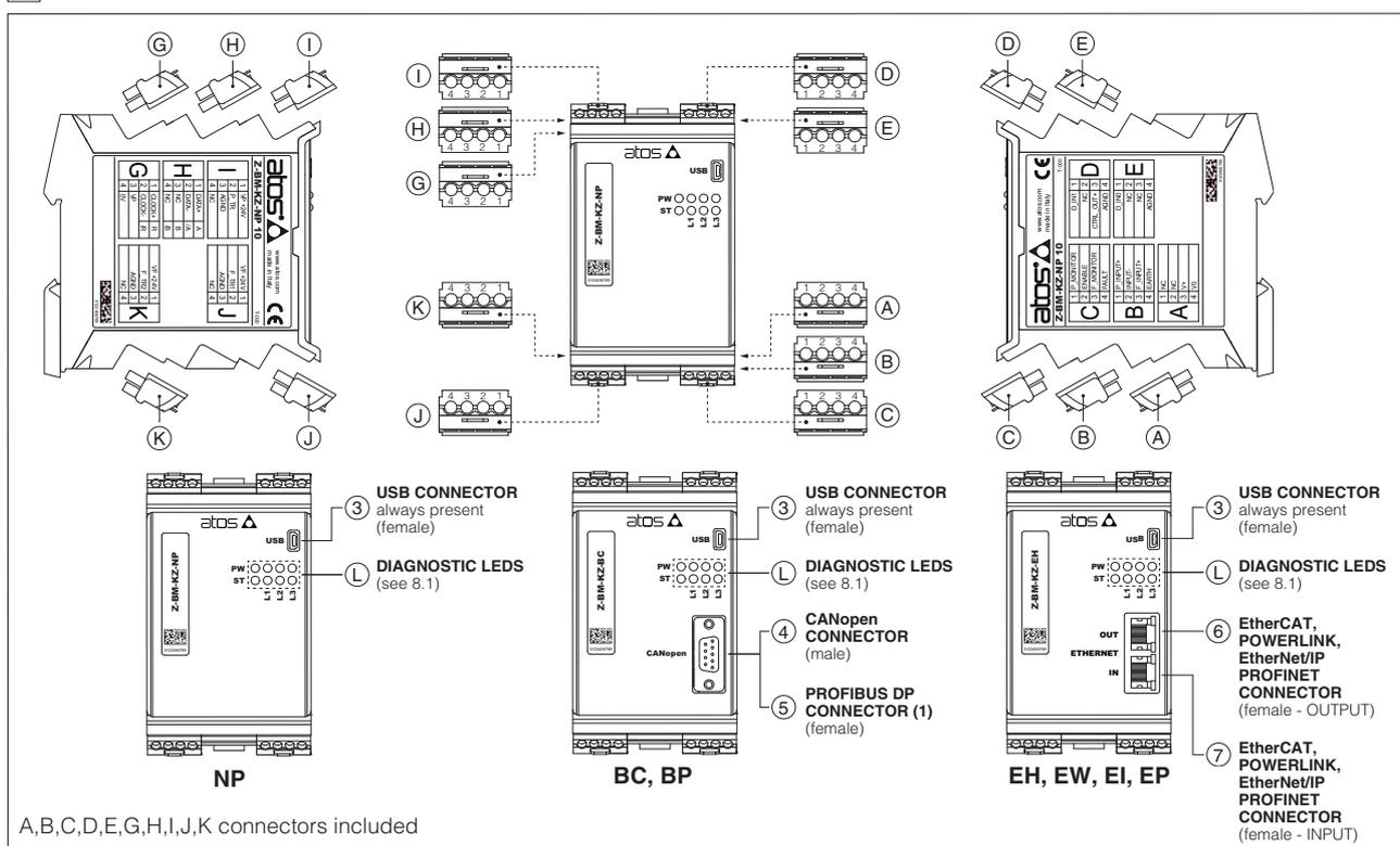
(1) To interface with Siemens 6ES7972-0BA12-0XA connector, it is mandatory to use also one of the following adapters to avoid interference with the USB connector: DG909MF1 - the connector will be oriented upwards; DG909MF3 - the connector will be oriented downwards
