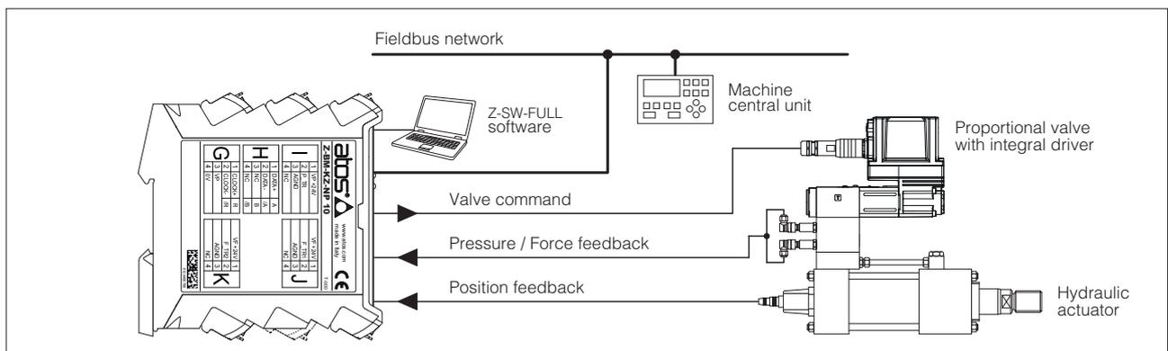
**Note:** block diagram example for alternated position/force control, with fieldbus interface
