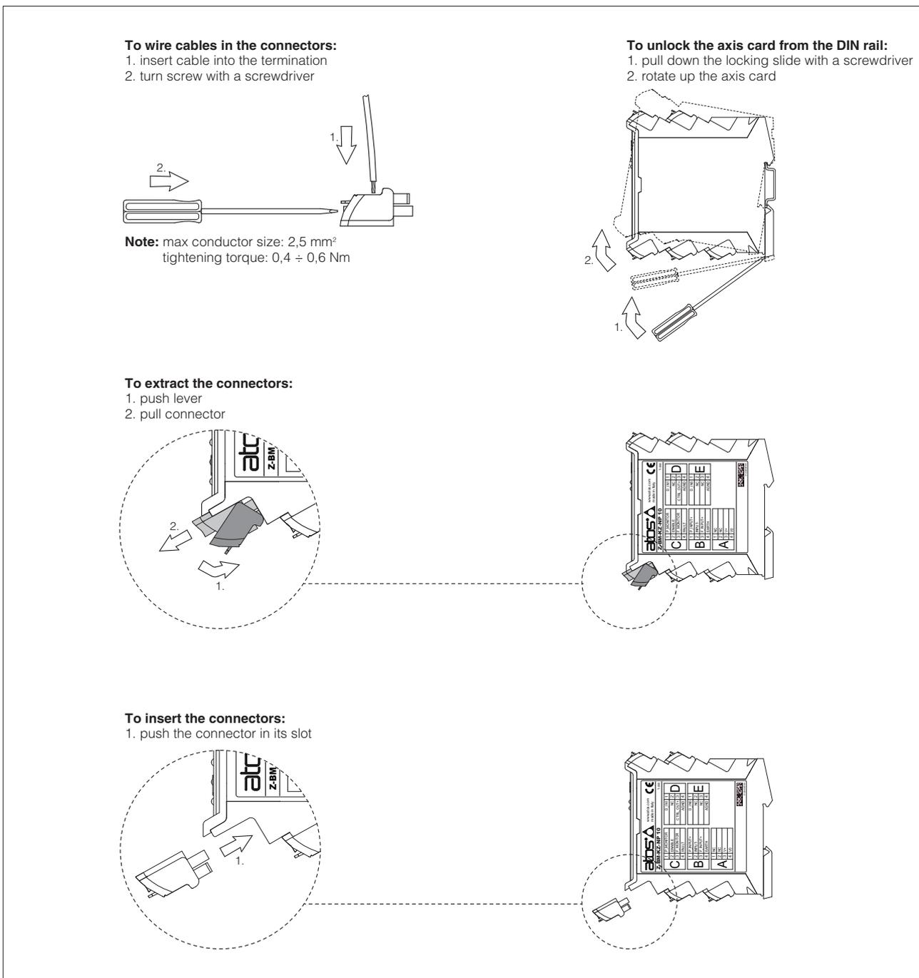
**Note:** all connectors are supplied with a mechanical coding. This feature ensures a unique insertion of each connector in the own slot (eg. connector A can not be inserted into connector slot of B,C,D,E,G,H,I,J,K)
