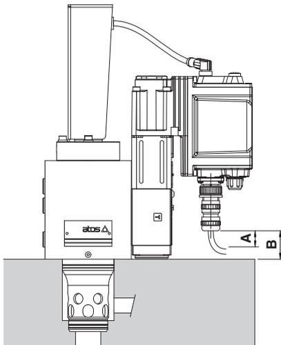
**A** = 15 mm space to remove the 7 or 12 pin main connectors
