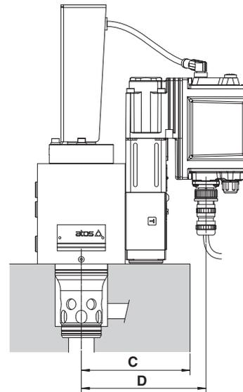
**C** = Max manifold dimension to avoid interference with the main connector, see below table
