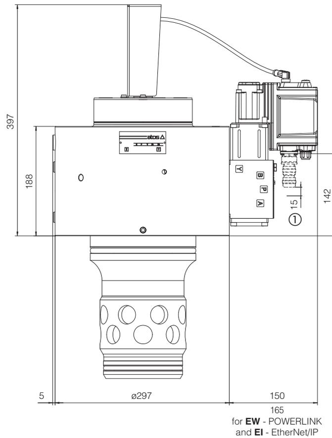
① Space to remove the 7 or 12 pin main connector. For main and communication connectors see section 11, 12
