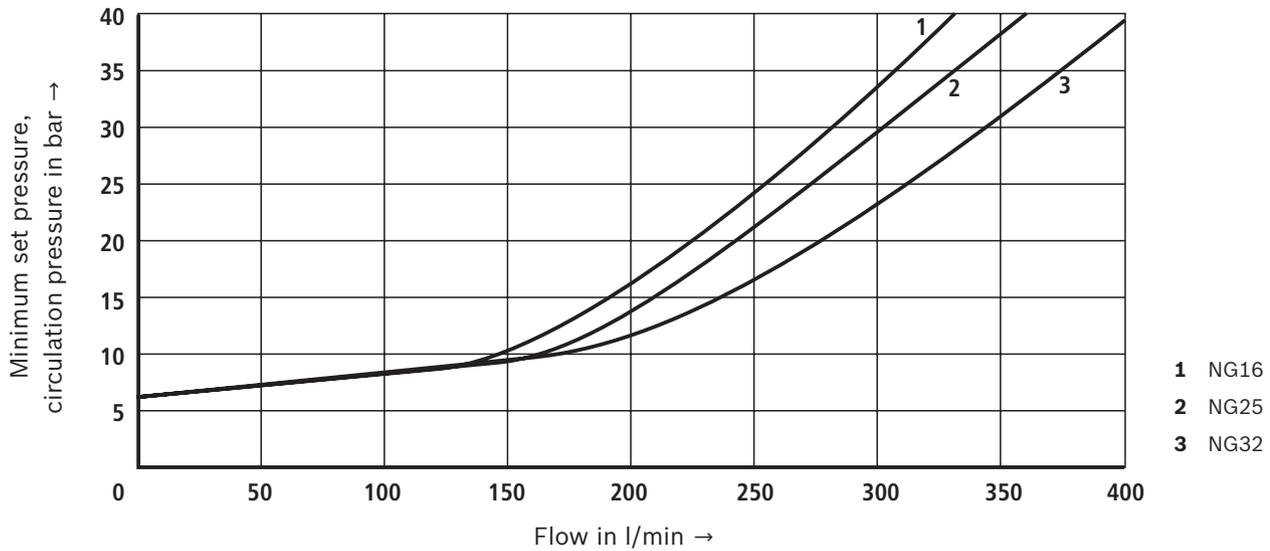
**Minimum set pressure and circulation pressure dependent on the flow <sup>1)</sup>**
