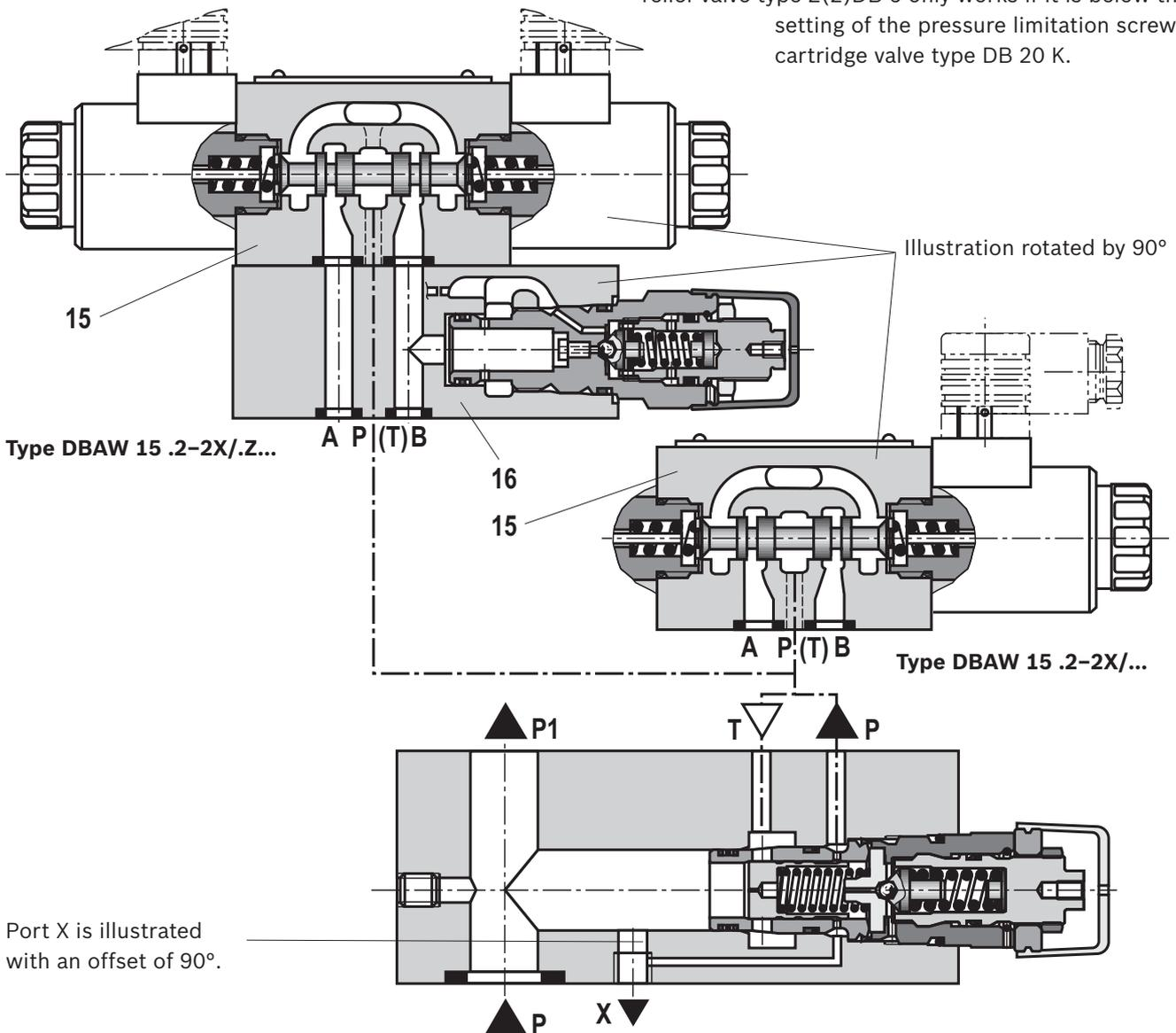
**Function, sections:** Type DBAE(E)... and DBAEA...
