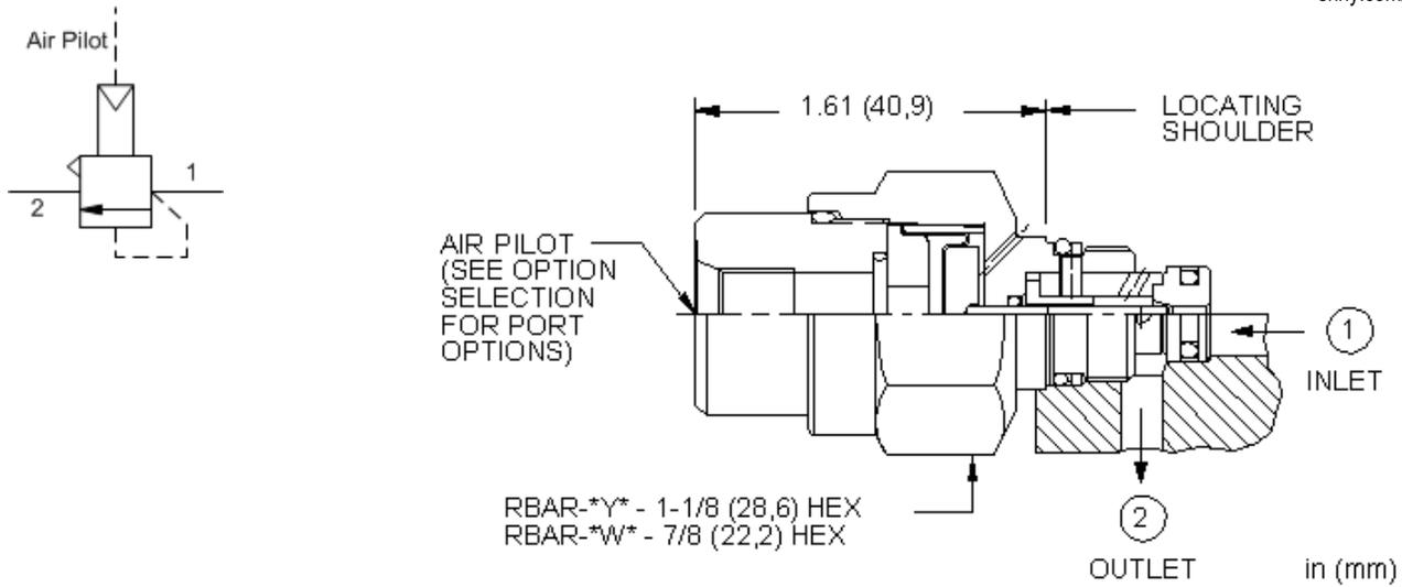
Two-port, pilot-stage, air-controlled, direct-acting relief cartridges are normally closed pressure regulating valves. When the pressure at port 1 (inlet) is sufficient to overcome the force due to the air signal, a flow path is opened from port 1 to port 2 (tank). These cartridges are designed for pilot flow applications and utilize Sun's T-8A cavity so they can be used in conjunction with Sun's pilot-operated, main-stage valves.
