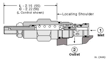
Direct-acting relief cartridges are normally closed, pressure-limiting valves used to protect hydraulic components from pressure transients. When the pressure at the inlet (port 1) reaches the valve setting, the valve starts to open to tank (port 2), throttling flow to limit the pressure rise. These valves are smooth and quiet, essentially zero leak, dirt tolerant, immune to silting and are very fast.
