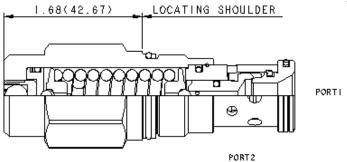
Non-adjustable direct-acting relief cartridges are normally closed, pressure-limiting valves used to protect hydraulic components from pressure transients. When the pressure at the inlet (port 1) reaches the valve setting, the valve starts to open to tank (port 2), throttling flow to limit the pressure rise. These valves are smooth and quiet, essentially zero leak, dirt tolerant, immune to silting and are very fast.
