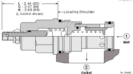
Kick-down relief cartridges act similar to a circuit breaker in an electrical system. The valves will kick completely open and remain open once the pressure at the inlet (port 1) exceeds the valve settting, creating an unrestricted flow path from port 1 to tank (port 2). The valve remains open as long as the pressure at port 1 exceeds the pressure at port 2. To reset the valve, flow from port 1 to port 2 must cease and pressure at port 2 must be equal to or greater than the pressure at port 1.
